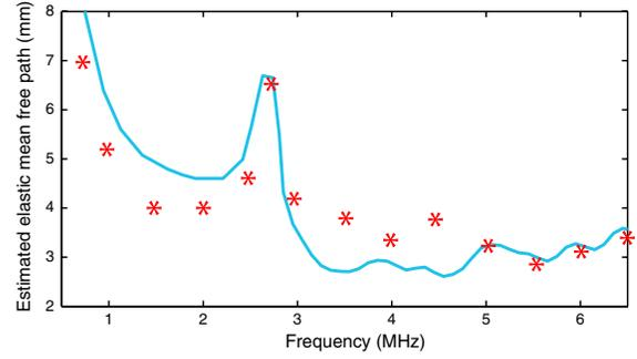
FIG. 3 (color online). Evolution with frequency of the reconstructed elastic mean free path. The reconstruction is done, according to Eq. (12), using convergence criterion. The red asterisks represent a theoretical prediction for a Gaussian distribution of radii [17] (mean radius 0.4 mm, standard deviation 8 mm).
