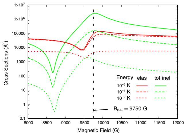
FIG. 2 (color online). Elastic (red) and total inelastic (green) cross sections for resonance 1 in  $\text{He} + \text{O}_2$  as a function of magnetic field at collision energies of  $10^{-6} \text{ K}$  (solid lines),  $10^{-4} \text{ K}$  (dashed lines), and  $10^{-2} \text{ K}$  (dotted lines).
