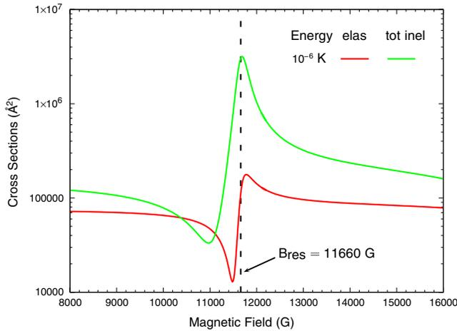
FIG. 3 (color online). Elastic (red) and total inelastic (green) cross sections for resonance 2 in He + O<sub>2</sub> as a function of magnetic field at collision energy 10<sup>-6</sup> K.
