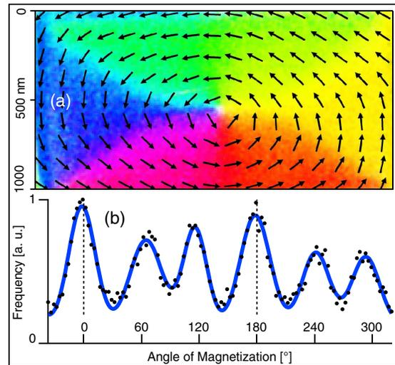
FIG. 6 (color online). Magnetization orientation of one single element from the array of Fig. 5. (a) shows a color (arrow) plot of the magnetic microstructure. The magnetization orientation was calculated from the SEMPA images. For easier understanding, arrows are given which show the direction of magnetization. (b) is the frequency of magnetization versus angle for the element shown in (a).
