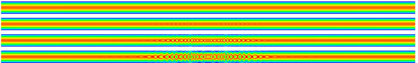
FIG. 1 (color online). Contour plots of the current density showing the time evolution of an SP current sheet for S = 10^8 . The times shown are, from top to bottom, t = 0.20\tau_A , t = 0.40\tau_A , t = 0.45\tau_A and t = 0.50\tau_A . The domain shown is -\delta_{\text{SP}} \leq x \leq \delta_{\text{SP}} (inflow direction, vertical), and -0.12L \leq y \leq 0.12L (outflow direction, horizontal), where \delta_{\text{SP}} \simeq 10^{-4} is the SP layer width and L = 1 is the (half-)length of the current sheet (see text; only the central half of the simulation box is shown).
