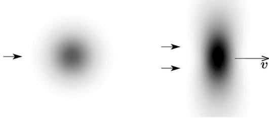
FIG. 3. The energy density around vortex cores moving at  $v = 0.45\sqrt{\frac{\mu}{M}}$ , with rotationally symmetric interaction parameters (see text). These profiles are obtained from numerical steady-state solutions to the two-dimensional Gross-Pitaevskii equation, Eq. (10). Blacker regions have greater energy densities. The small arrows indicate the roots of  $\psi_1$  and  $\psi_{-1}$ .
