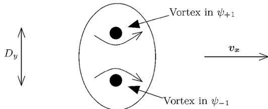
FIG. 2. Seeing the momentum of a spin vortex. The phases of  $\psi_{\pm 1}$  increase in the directions of the arrows. The component vortices are pulled apart by the lift force to a distance  $D_y \propto p_x$ . The phase locking produced by the spin-dependent interaction limits the stretching, since the phase  $\lambda$  is nonzero over the region indicated by the ellipse.
