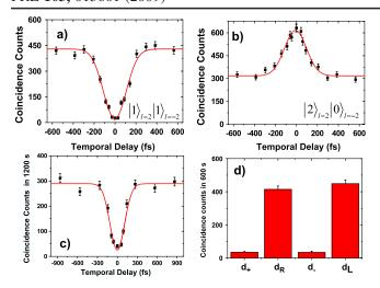
FIG. 4 (color online). (a) Coincidence counts between  $[D_A, D_B]$  versus the temporal delay  $t_d$ , for the state  $|\Psi_{\text{out}}\rangle$ . The continuous line shows the best fit of the experimental data. (b) Coincidence counts  $[D_A, D_{A'}]$  versus  $t_d$ . (c) Coincidence counts  $[D_A, D_B]$  versus  $t_d$   $[V = (0.91 \pm 0.01)]$  for the state  $|\Phi_{\text{out}}\rangle$ . (d) Coincidence counts  $[D_A, D_{A'}]$  in different OAM bases.
