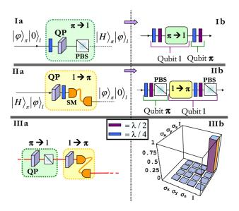
FIG. 3 (color online). (I),(II) Schematic representation of the two transferrer devices based on the q plate (QP). (III) (a) Double transfer  $\pi \to l \to \pi$  and (b) experimental real part of the matrix  $\chi$  represented in the Pauli operator basis, the imaginary elements are  $\approx 0$ .
