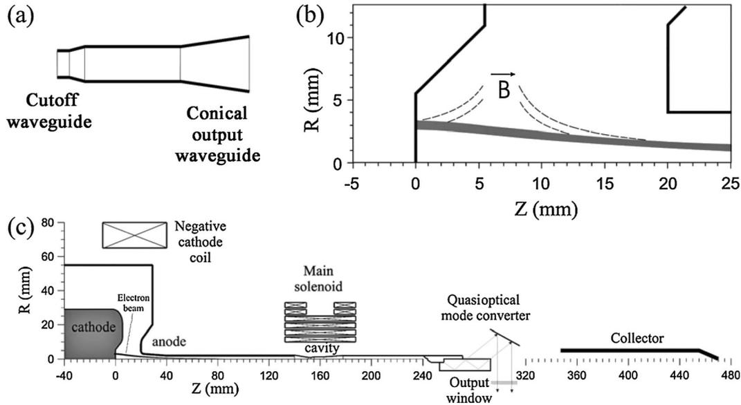
FIG. 1. The 1-THz third-harmonic LOG: cavity (a), cusp gun (b), and general scheme (c).
