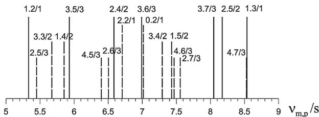
FIG. 2. The spectrum of potentially exciting cavity modes  $TE_{m,p}$  (contracted notations  $m.p/s$  are used for the excitation at the  $s$ th cyclotron harmonic; the value  $v_{m,p}/s$  is proportional to the resonant magnetic field).
