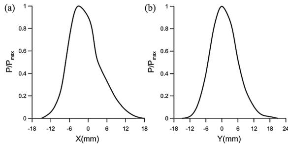
FIG. 6. Horizontal (a) and vertical (b) distributions of radiated power at a distance of 160 mm from the output window for an operating frequency of 1 THz.
