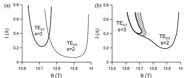
FIG. 3. Calculated (a) and experimentally observed (b) regions of excitation for the operating third-harmonic mode  $TE_{3,7}$  and closest spurious second-harmonic mode  $TE_{2,5}$  in the 1-THz LOG (two-frequency generation was observed in the shaded area between the regions of the  $TE_{3,7}$  and  $TE_{2,5}$  modes).
