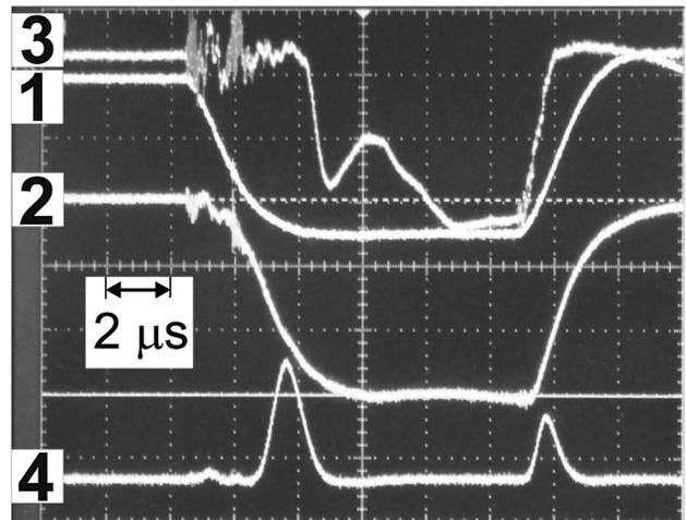
FIG. 5. Oscilloscope traces: pulse voltage (1) and current (2), detector signals for the  $TE_{3,7}$  (3) and  $TE_{2,5}$  (4) modes.
