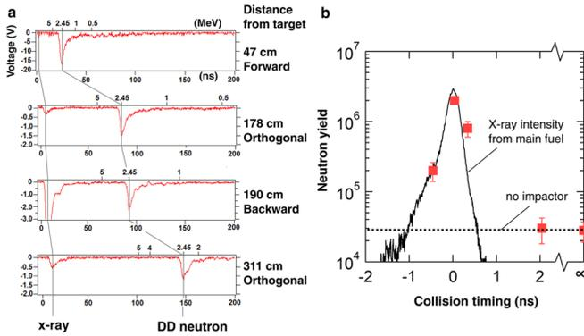
FIG. 4 (color online). (a) Time-of-flight signals of neutron emission. Neutrons were detected at different flight distances and orientations with respect to the acceleration direction of the impactor. (b) Neutron yield as a function of collision timing.
