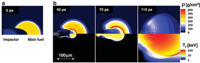
FIG. 1 (color). (a) Initial configuration of the impactor and the main fuel. (b) Snapshots of density and temperature distributions obtained from the simulation. The thin white lines indicate the impactor outer boundary. At a time of 110 ps, ignition and burn can be observed with temperatures  $>30$  keV.
