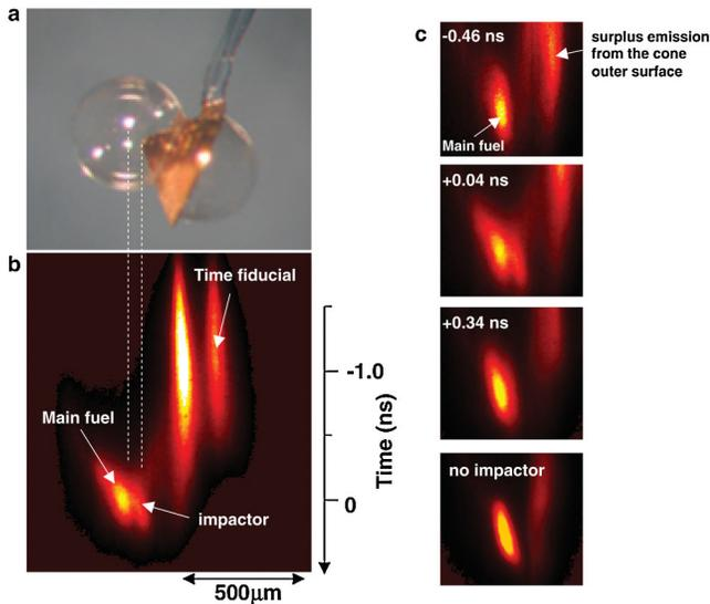
FIG. 3 (color). (a) Integrated target used for the impact ignition experiment. (b) Streaked x-ray image showing the collision of the impactor with the precompressed main fuel. (c) X-ray images at the center for four different times of the impactor collision with respect to the maximum compression.
