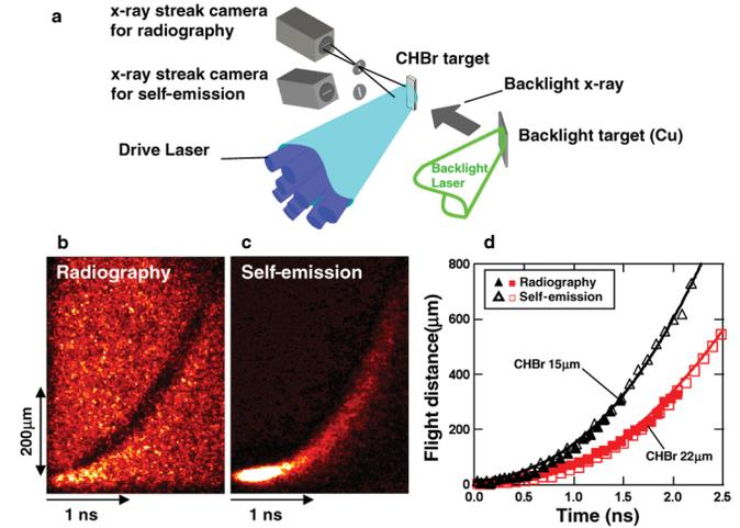
FIG. 2 (color). (a) The setup used for the foil trajectory measurement. The time origin of this experiment is defined as the time of the first half maximum of the laser. (b) Time-resolved x-ray radiography of a brominated polystyrene foil target moving to the target normal. (c) Time-resolved x-ray emission image from the target. (d) Compiled data of the flight distance vs time.
