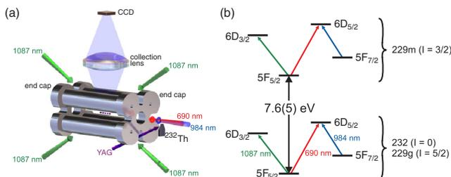
FIG. 1 (color online). (a) Schematic of linear rf Paul trap and  $^{232}\text{Th}$  sample. (b) Lowest electronic energy levels of  $\text{Th}^{3+}$ .
