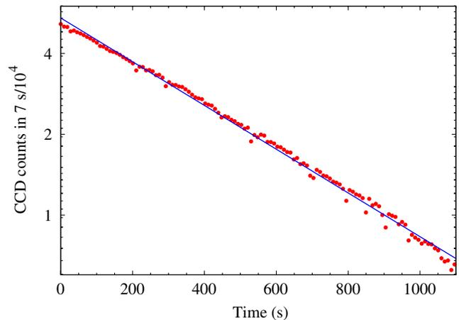
FIG. 4 (color online). Measured fluorescence signal from the 984 nm transition of a cold  $\text{Th}^{3+}$  cloud. The 984 nm field was detuned  $\sim 1$  MHz below resonance, while the 690 nm field was on resonance to avoid optical pumping into the  $5F_{5/2}$  state. The exponential fit gives a  $1/e$  lifetime of 646(10) s. The relatively short ion lifetime is attributed to charge exchange collisions with residual buffer gas impurities.
