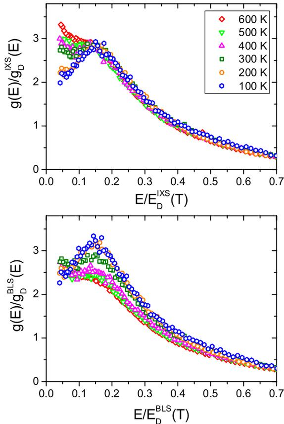
FIG. 3 (color online). Upper panel: VDOS in Debye units, where the Debye energy is determined starting from the high-frequency IXS values of the sound velocities. Lower panel: VDOS in Debye units, but with Debye energy values calculated starting from the BLS data, and thus affected by anharmonic effects.
