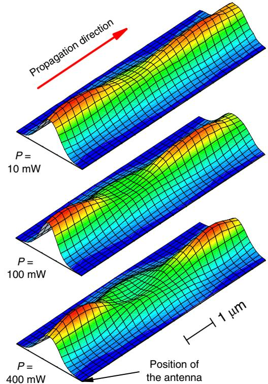
FIG. 2 (color online). Measured maps of SW intensity in the continuous-wave excitation regime for different powers  $P$  applied to the antenna. The maps have dimensions of 2.4 by 7  $\mu\text{m}$ . Spatial decay is numerically compensated.  $F = 8.8$  GHz.  $H = 830$  Oe.
