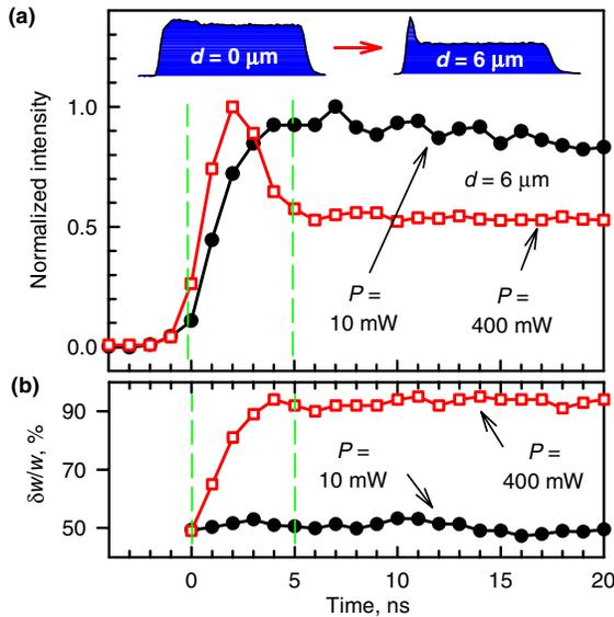
FIG. 5 (color online). (a) Waveforms of the leading part of SW pulse detected at  $d = 6 \mu\text{m}$  for the linear ( $P = 10$  mW) and the strongly nonlinear ( $P = 400$  mW) cases. Inset—waveforms of the nonlinear ( $P = 400$  mW) SW pulse detected  $d = 0$  and  $6 \mu\text{m}$ . (b) Temporal dependences of the modulation depth  $\delta w/w$  for the linear and the strongly nonlinear cases.
