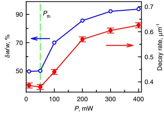
FIG. 4 (color online). Dependences of the modulation depth of SW beam  $\delta w/w$  and the mean decay rate of SW intensity on the excitation power  $P$ .  $P_{\text{th}}$  denotes the threshold power necessary for the appearance of the self-modulation and the nonlinear damping phenomena.
