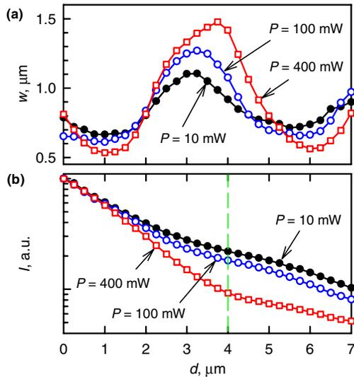
FIG. 3 (color online). (a) width of SW beam  $w$  as a function of the propagation distance  $d$  for different excitation powers  $P$ . (b) spatial variation of the integral of SW intensity over transverse sections  $I$ , characterizing the spatial decay of SWs at different  $P$ . The data are normalized at  $d = 0$ . Note the logarithmic scale of the vertical axis.  $F = 8.8$  GHz.  $H = 830$  Oe.
