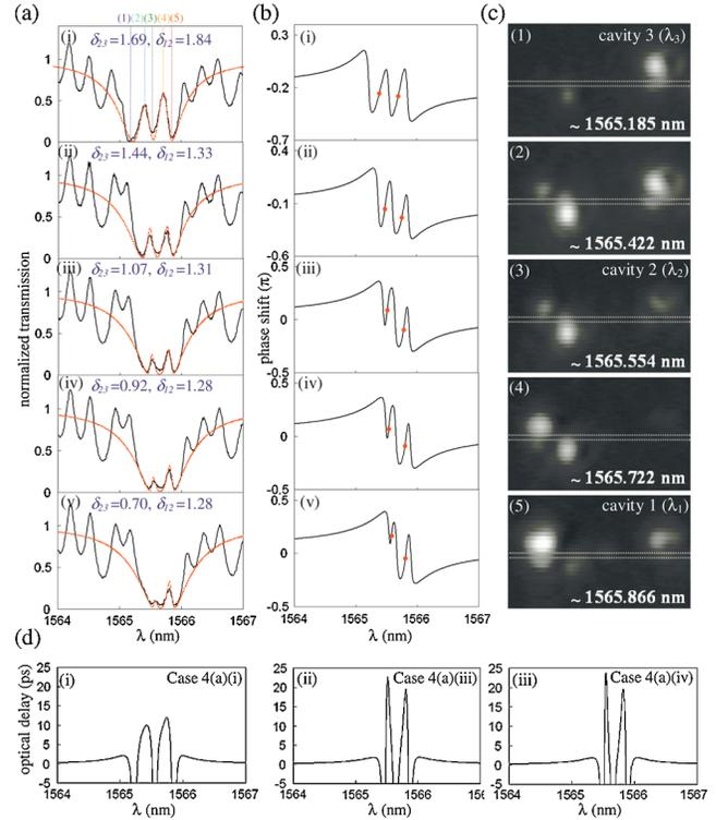
FIG. 4 (color online). (a) Measured and theoretical transmission line shapes with various detuning  $\delta_{12}$  and  $\delta_{23}$  for sample 4. (a.i) Denotes the frequencies where the radiation images are collected. (b) Corresponding theoretical transmission phase shift. (c) Top-collected radiation images for various detunings. (d) Calculated optical delays for double EIT-like peaks.
