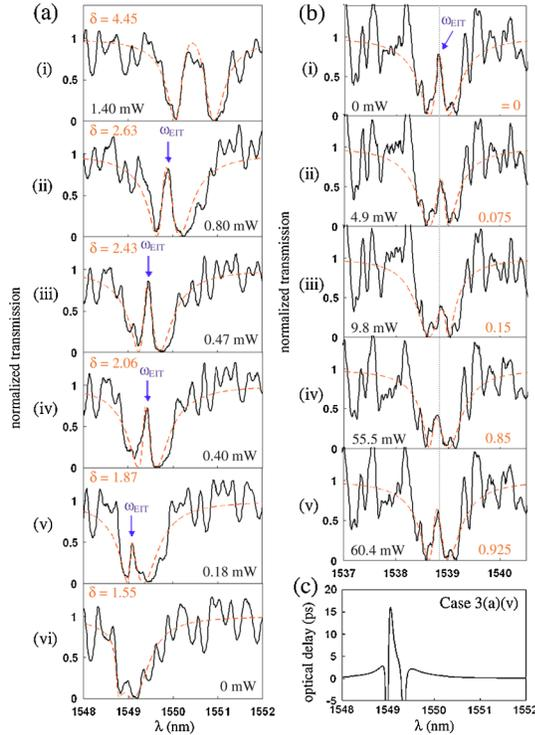
FIG. 3 (color online). (a) Measured and theoretical transmission line shapes with various detuning  $\delta$  for sample 2,  $L = 10a$ . (b) Measured and theoretical transmission line shapes with various phase difference  $\Delta\phi$  at  $\delta = 1.92$  for sample 3,  $L = 142a$ . The dotted gray lines show the position of the EIT-like transparency peak for  $\Delta\phi = 0$ . (c) Calculated optical delay.
