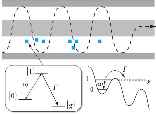
FIG. 1 (color online). Detector design. Sketch showing a one-dimensional waveguide (gray bars) coupled to a set of three-level absorbers (squares) in arbitrary positions. The microwave field (dashed line) excites coherently the state  $|0\rangle$  to the upper state  $|1\rangle$ , which decays onto a long-lived stable state. An analogous setup uses current-biased Josephson junctions, in which a washboard potential confines two metastable states that can decay into a continuum of current states.
