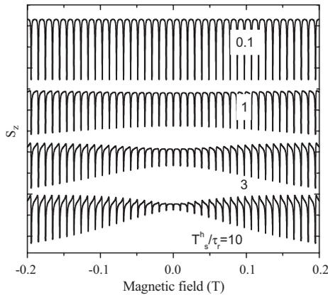
FIG. 2. Calculated RSA spectra for a homogeneous spin ensemble excited at trion resonance, based on Eqs. (3)–(6).  $\delta = 10$  ps,  $|g_e| = 0.555$  (determined from RSA peak distance),  $\Delta g_e = 0$ ,  $T_s^e = 55$  ns, and  $\tau_r = 120$  ps for different ratios  $T_s^h$  to  $\tau_r$ , given at each curve.
