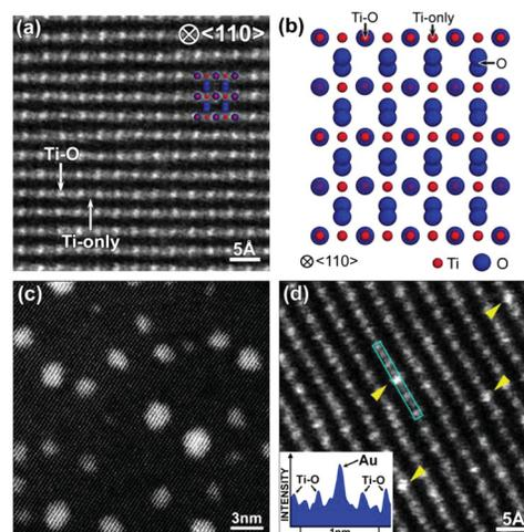
FIG. 1 (color). (a) Atomic-resolution HAADF STEM image of a rutile TiO<sub>2</sub> single crystal observed from  $\langle 110 \rangle$  direction. (b) The corresponding crystal structure model. (c) Typical HAADF STEM image of Au nanoparticles deposited on a TiO<sub>2</sub> (110) surface. (d) HAADF STEM image of single Au atoms on the TiO<sub>2</sub> (110) surface. Inset shows the image intensity profile across a single Au atom, showing strong image intensity on the Ti-O columns.
