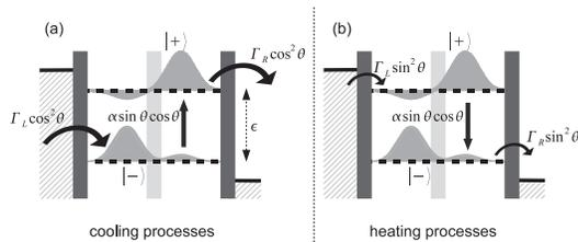
FIG. 3. Dominant cooling (a) and heating (b) processes in the parameter region of optimal cooling in Fig. 2. States  $|-\rangle$  and  $|+\rangle$  denote the bonding and antibonding states at frequency difference  $\epsilon = \sqrt{\Delta^2 + 4T_c^2}$ . The rates are reported in the new basis, with  $\tan\theta = 2T_c/(\Delta + \epsilon)$ . For  $\Delta > 0$ , then  $\tan^2\theta < 1$  and the processes in (a) are faster, so that the resonator is cooled.
