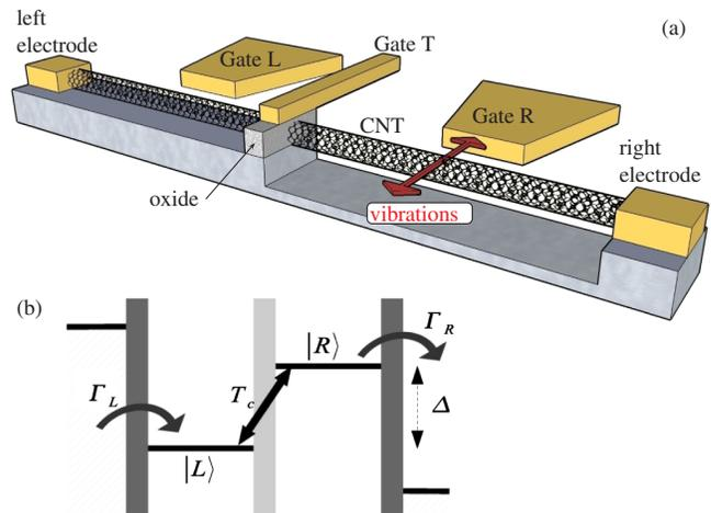
FIG. 1 (color online). (a) Sketch of the double quantum dot, carbon-nanotube (CNT) device. The dot on the right is suspended, and mechanically oscillates. (b) The single-electron levels  $|L\rangle$  and  $|R\rangle$ , at (tunable) frequency difference  $\Delta$ , are coherently coupled with tunneling rate  $T_c$ .
