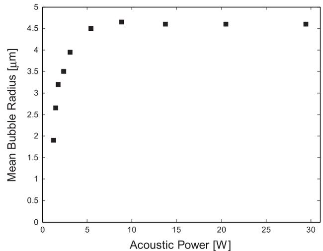
FIG. 2. Bubble radii (mean of the size distribution) under 1056 kHz sonication as a function of acoustic power.
