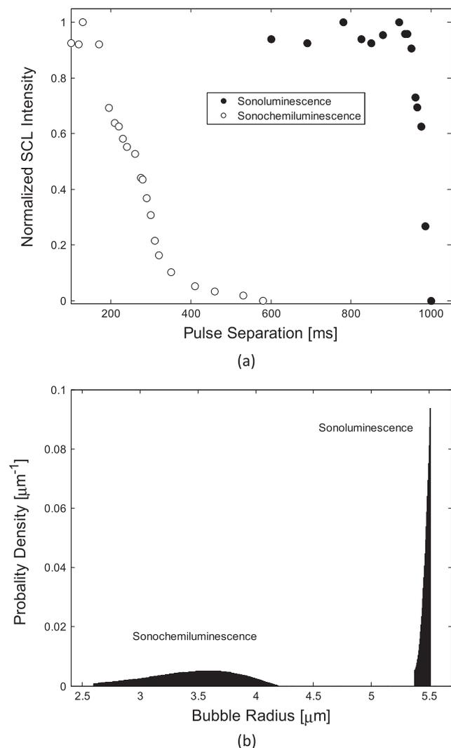
FIG. 3. (a) Normalized sonochemiluminescence intensity from luminol and sonoluminescence intensity as a function of pulse separation (with a constant pulse time of 4 ms) at 575 kHz and (b) the bubble-size distributions determined from the sonochemiluminescence and sonoluminescence data. The acoustic power in (a) and (b) was  $2.8 \pm 0.5$  W.
