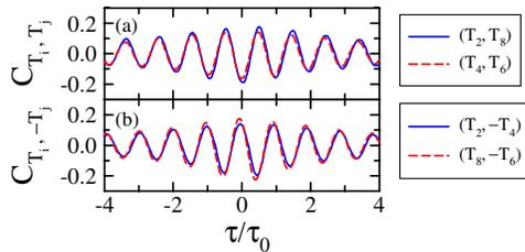
FIG. 4 (color online). Temperature cross-correlation functions measured in-fluid at midheight plane.
