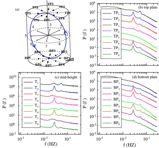
FIG. 1 (color online). (a) Sketch of the convection cell and thermistor configurations. Power spectra of temperatures measured by thermistors (b) embedded in the top plate at positions TP1 to TP8 (from top to bottom); (c) at midheight positions T1 to T8 in the bulk fluid; and (d) embedded in the bottom plate at positions BP1 to BP8. For clarity, each data set is shifted up from its lower neighbor by a factor of 20.
