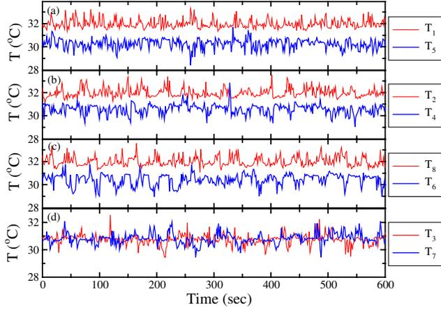
FIG. 3 (color online). Time traces of the temperature measured at the midheight plane by thermistors  $T_1$  to  $T_8$ . For clarity,  $T_1$ ,  $T_2$ , and  $T_8$  are shifted up by  $1^\circ\text{C}$ .
