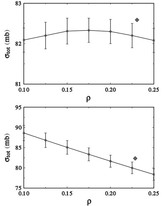
FIG. 3. The size of  $\sigma_{\text{tot}}$  obtained by fitting the simulated data assuming a fixed value of  $\rho$  at  $\sqrt{s} = 2 \text{ TeV}$  with  $\mathcal{L}$  fixed at the input value (upper panel) and with free  $\mathcal{L}$  (lower panel); the diamond gives the true value of  $\sigma_{\text{tot}}$  and  $\rho(s, 0)$ .
