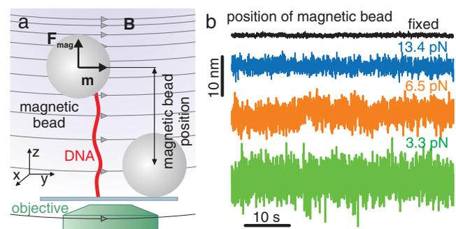
FIG. 1 (color). (a) Schematics of the experimental setup. (b) Time traces of the  $z$  position of the magnetic microsphere at different forces. The black trace is for a fixed microsphere.
