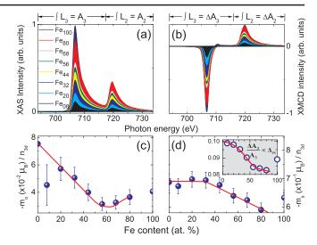
FIG. 3 (color online). (a) Background subtracted Fe  $L_{2,3}$  edge XAS. (b) Corresponding XMCD spectra. (c) Orbital moment per hole,  $\frac{m_0}{n_{3d}}$ . (d) Spin moment per hole,  $\frac{m_0}{n_{3d}}$ . Inset shows  $\frac{\Delta A_3}{A_3} \propto \Delta_{\rm ex}$  [27]. Fe $_0$  represents Co $_{80}$ B $_{20}$  measured at the Co  $L_{2,3}$  edges. Lines in (c) and (d) are guides to the eye.
