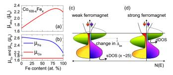
FIG. 1 (color online). Schematic representation of the S-P behavior for  $\text{Co}_{100-x}\text{Fe}_x$ : (a) S-P curve of  $\mu_{\text{alloy}}$  [5]. (b) Known trend of the element-specific Co and Fe moments [6]. DOS of (c) weak and (d) strong ferromagnets.
