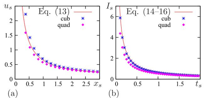
FIG. 2 (color online). Comparison of analytical predictions with numerical simulations. (a) Strength-extent curves for rectangular initial conditions. (b) Strength-duration curves for point stimulation. Red solid lines: Analytical approximations, (13) for (a) and (14)–(16) for (b). Blue stars (“cub”): Numerical results for cubic kinetics (2). Magenta diamonds (“quad”): Numerical results for quadratic kinetics (12).
