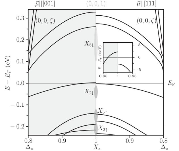
FIG. 1. Quasiparticle band structure along the  $\Delta$  line around the  $X_z$  point of the Brillouin zone for magnetic-moment directions  $\vec{\mu} \parallel [001]$  and  $\vec{\mu} \parallel [111]$ . The inset shows an enlarged view of the band structure around the Fermi energy which displays the additional hole ellipsoid for  $\vec{\mu} \parallel [001]$  more clearly.
