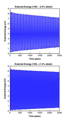
FIG. 1 (color online). Top: External energy time history of oscillating  $10.85 \times 1.45 \times 1.45$  nm copper nanowire at 10 K, 2.5% compressive strain. Bottom: External energy time history of oscillating  $10.85 \times 1.45 \times 1.45$  nm copper nanowire at 10 K, 1.5% tensile strain.
