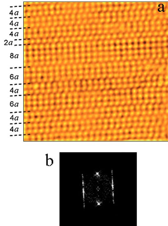
FIG. 4 (color online). (a) STM image obtained at 77 K on top of Ga(001) island on Si(111). The image sizes are  $215 \times 200 \text{ \AA}^2$ . The domain boundaries are indicated by dashed lines. The image was obtained at  $I = 0.2$  nA and  $V_{\text{tip}} = -500$  mV. (b) The Fourier transform of STM image in (a).
