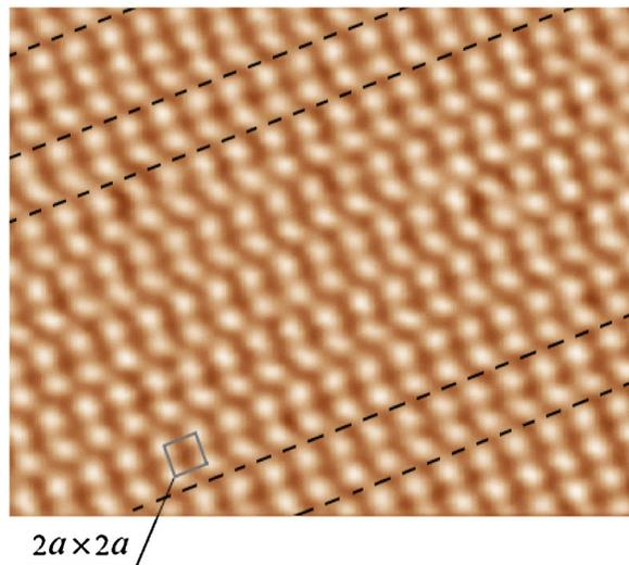
FIG. 2 (color online). STM image obtained at 77 K on top of Ga(001) island on Si(100). The image sizes are  $155 \times 120 \text{ Å}^2$ . The electronic superlattice, whose periodicity is  $9.0 \times 9.0 \text{ Å}^2$ , is composed of unidirectional stripe domains. Some of the domain boundaries are indicated by dashed lines. The image was obtained at  $I = 0.2 \text{ nA}$ ,  $V_{\text{tip}} = -500 \text{ mV}$ .
