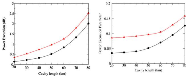
FIG. 4 (color online). Evolution of the power excursion (left panel) and  $\delta P$  parameter (right panel) vs cavity length for 0 dBm total signal power. Triangles, 20 nm bandwidth; circles, 10 nm bandwidth.
