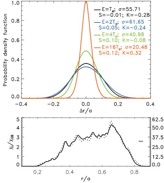
FIG. 2 (color). *Lower panel:* Radial profiles for thermal ion heat conductivity  $\chi_i$  and ITG intensity of fluctuating potential  $I = (\epsilon \delta \phi / \rho^* T_e)^2$ . *Upper panel:* Probability density functions of the radial excursion  $\Delta r/a$  for particle energy  $E/T_e = 1$  (black), 2 (blue), 4 (green), 16 (orange).  $\sigma$ ,  $S$ , and  $K$  are the standard deviation (in unit of  $\rho_i$ ), skewness, and kurtosis, respectively.
