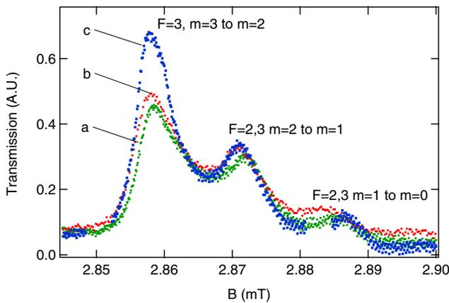
FIG. 2 (color online). ESR spectra of  $^{85}\text{Rb}$  for full flux [(a): green] and 19% of full flux [(b): red] and no beam [(c): blue] at LANSCE. The polarizations are  $P_A = 0.78, 0.81,$  and  $0.90$ , respectively. The relative uncertainties, estimated to be 1%–2%, are limited by the signal-to-noise ratio of the ESR measurements.
