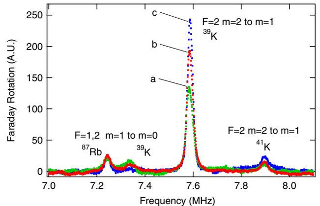
FIG. 3 (color online). ESR spectra of  $^{39,41}\text{K}$  and  $^{87}\text{Rb}$  for full flux [(a): green] and 8.5% of full flux [(b): red] and no flux [(c): blue] at ILL. The polarizations are  $P_A = 0.83, 0.90,$  and  $0.98$ , respectively.
