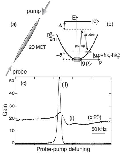
FIG. 1. (a) Schematic indicating the pump and probe beams used for the RIR, where MOT is the magneto-optic trap. (b) The energy levels relevant to the RIR. (c) Absorption spectrum of a probe beam around the RIR for longitudinal optical depth of  $\sim 10$  (i) and  $\sim 40$  (ii).
