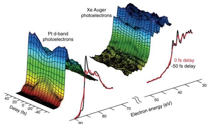
FIG. 3 (color). Photoelectron spectra from Xe/Pt(111) as a function of time delay. Negative time delays denote that the SXR pump pulse arrives after the IR probe pulse. The time evolution of the redistribution of electrons due to the IR dressing at the Pt  $d$  band and at the Xe Auger photoelectron peaks can be observed. The spectra shown in the lineouts correspond to the photoelectron spectrum at zero (red) and at  $-50$  (black) fs time delay between the SXR and the IR pulses.
