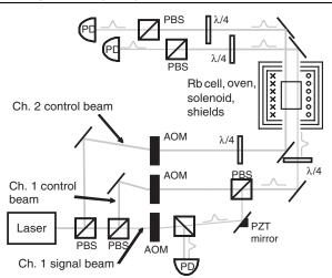
FIG. 2. Schematic of the apparatus used in the coated cell slow light beam splitter experiments. (*See text for details.*)
