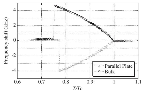
FIG. 1. Frequency shift from the Larmor frequency observed between parallel plates (triangles) and in bulk (circle) as a function of temperature normalized by  $T_c$ . Frequency shifts disappeared in lower temperature because of the transition to the superfluid B phase.
