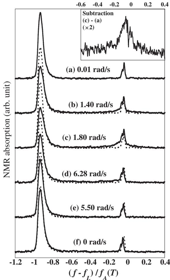
FIG. 2. NMR spectra at 0.01, 1.40, 1.80, 6.28, 5.50, and 0 rad/s. All spectra were measured at  $0.81T_c$  in the order of showing up to down. The superfluid was cooled at  $H = \Omega = 0$  during the superfluid transition. For the spectra of (b)–(f), the first spectrum (a) is shown as a dotted line for reference. The inset is an enlarged view of the satellite signal obtained from a subtraction between data at 1.8 rad/s and at 0.01 rad/s.
