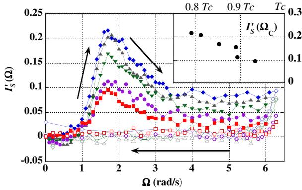
FIG. 5 (color online). The temperature dependence of  $I'_s(\Omega)$  at 0.79 (blue diamonds), 0.81 (gray triangles), 0.85 (green inverted triangles), 0.89 (purple circles), and 0.93  $T_c$  (red squares). All measurements were done after warming above  $T_c$  and cooling  $H = \Omega = 0$  during the superfluid transition. The filled (open) symbols are taken in acceleration (deceleration). The inset shows  $I'_s(\Omega_c)$  vs  $T/T_c$ .
