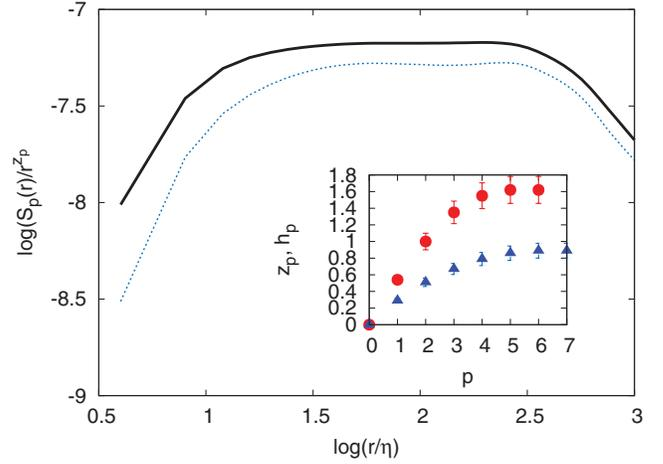
FIG. 3 (color). Compensated structure functions of the density  $D_6(r)r^{-z_6}$  (solid line) and  $D_5(r)r^{-z_5}$  (dashed line). Inset: scaling exponents of the density (●) and entropy (▲) structure functions. Errors include both statistical fluctuations and the uncertainty in the fit to the inertial range.
