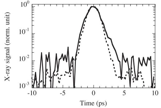
FIG. 2. Temporal profile of the x-ray pulse (with arbitrary origin). 275 Å average radius Ar clusters are irradiated by 2.0 mJ, 320 fs FWHM, linearly polarized laser pulse. Full line: x-ray measurement. Dashed line: 0.8 ps rms instrumental response as measured on the same setup with third harmonic generated from 40 fs laser pulses.
