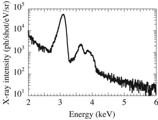
FIG. 1. X-ray emission spectrum recorded by the broadband spectrometer. 275 Å average radius Ar clusters are irradiated by 2.0 mJ, 320 fs FWHM, linearly polarized laser pulse. The laser intensity is  $7.5 \pm 2.5 \times 10^{15}$  W/cm<sup>2</sup>. 25 μm Be and six other filters, each composed by 6 μm Mylar and 0.3 μm Al, are set up in front of the detector.
