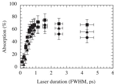
FIG. 4. Laser energy absorption measured in the cluster jet as a function of the laser pulse duration. Ar clusters with 180 Å (circles), 275 Å (squares) and 350 Å (triangles) average radius are irradiated by 2.0 mJ, linearly polarized laser pulses.
