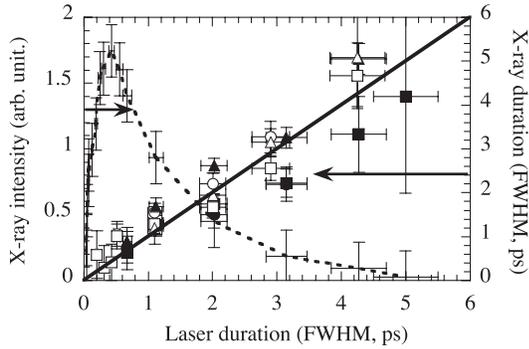
FIG. 3. X-ray emission duration measured as a function of the laser pulse duration. Ar clusters with 180 Å (circles), 275 Å (squares), and 350 Å (triangles) average radius are irradiated by 2.0 mJ, linearly (black) and circularly (white) polarized laser pulses. Full line: guiding line equating the x-ray pulse duration to the laser pulse duration. Dashed line: time-integrated  $K$ -shell x-ray emission from 275 Å Ar clusters.
