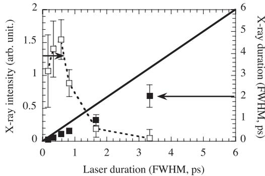
FIG. 5. Black squares: x-ray emission duration calculated as a function of the laser pulse duration from a 275 Å average radius Ar cluster. Full line: guiding line equating the x-ray pulse duration to the laser pulse duration. White squares and dashed line: time-integrated *K*-shell x-ray emission deduced from the calculation.
