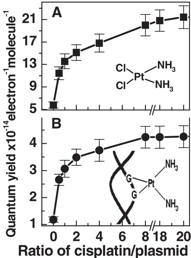
FIG. 2. Comparison of the yield of SSB (A) and DSB (B) as a function of different cisplatin to plasmid ratios. The yields were obtained from exposure curves of 5 ML cisplatin/plasmid mixture deposited on a tantalum substrate and bombarded with  $100 \pm 0.5$  eV electrons.
