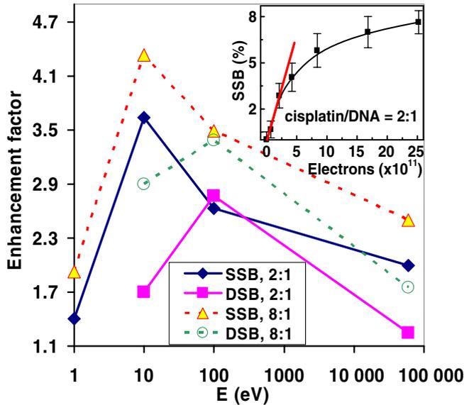
FIG. 1 (color online). Enhancement of damage arising from the bonding of 2 and 8 cisplatin molecules to DNA as a function of electron energy. The exposure response curve for production of SSB by 100 eV electrons is shown in the upper inset.
