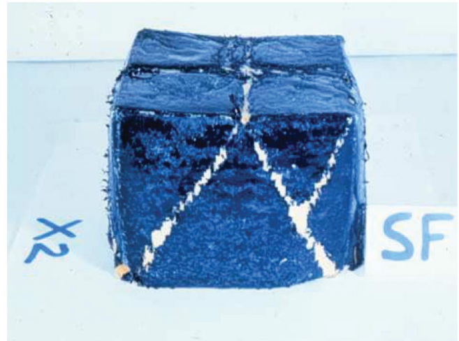
FIG. 1 (color). A dry dense sand cubic specimen ( 100 \times 100 \times 100 \text{ mm}^3 ) that was sheared by a triaxial test apparatus that can control three principal stresses independently. The specimen was surrounded by six rigid planes, and was deformed into a right-angled prism with confining pressure of 300 kPa.
