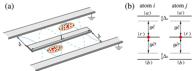
FIG. 1 (color online). (a) CPW cavity with stripline length  $L$  and electrode distance  $d$ . Ensembles of ground state atoms are trapped near the CPW surface within antinodes of the standing wave field. (b) Level scheme of excited Rydberg atoms  $i$  and  $j$  interacting nonresonantly with a common cavity mode.
