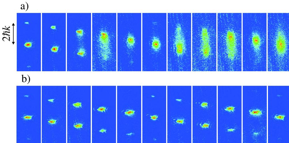
FIG. 1 (color online). Bloch oscillations from 0 to 4 ms, in steps of 0.4 ms, for a condensate with (a)  $100 a_0$  and (b)  $1 a_0$  scattering length. The picture shows absorption images of the cloud after release from the lattice. The expansion lasts 12.5 ms, and the scattering length is changed to  $-33 a_0$  only 3 ms before image acquisition.
