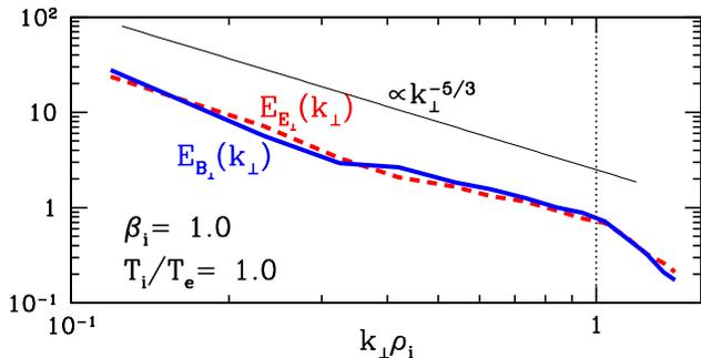
FIG. 2 (color online). Magnetic (solid line) and electric (dashed line) energy spectra in the MHD regime ( $k_\perp \rho_i < 1$ ). The box size is  $L_\perp/2\pi = 10\rho_i$ . Electron hypercollisionality is dominant for  $k_\perp \rho_i \geq 1$  (dotted line).
