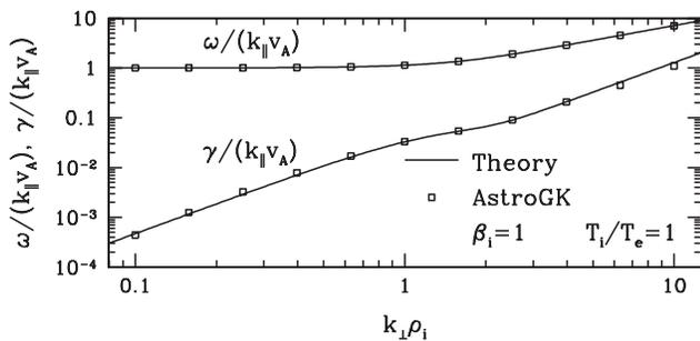
FIG. 1. Normalized frequencies  $\omega/k_{\parallel}v_A$  and damping rates  $\gamma/k_{\parallel}v_A$  vs normalized perpendicular wave number  $k_{\perp}\rho_i$  for a plasma with  $\beta_i = 1$  and  $T_i/T_e = 1$ . ASTROGK (squares) correctly reproduces the analytic results from the linear collisionless gyrokinetic dispersion relation (line) [8].
