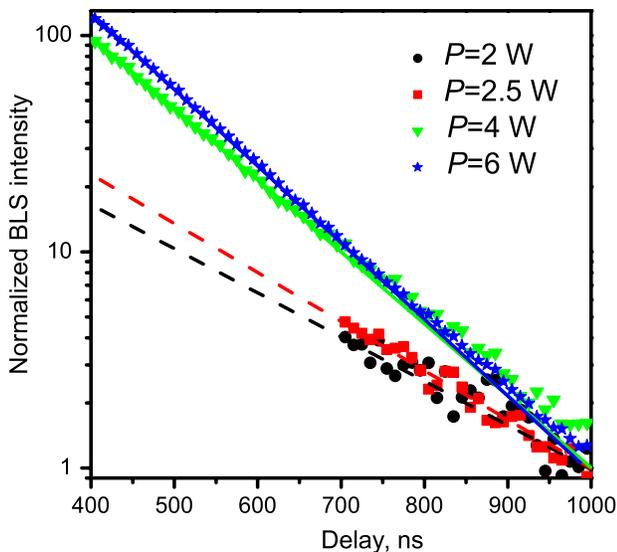
FIG. 2 (color online). Decay of the BLS intensity at the lowest magnon frequency  $f_{\min}$  after the formation of the overpopulated state is finished for different values of the pumping power, as indicated. Lines—best fit of the experimental points by the exponential decay function.
