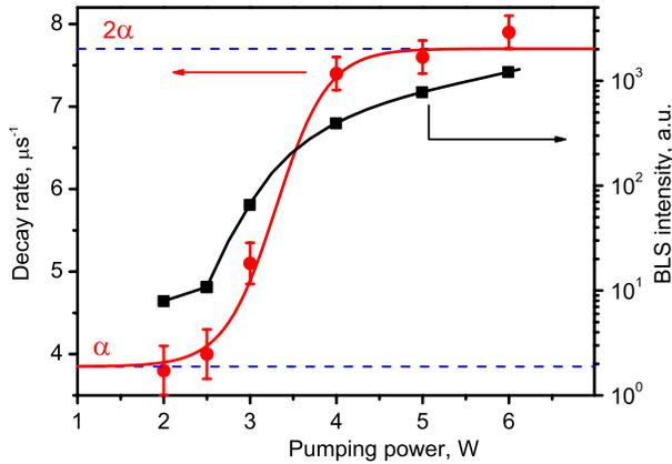
FIG. 3 (color online). Circles—dependence of the measured decay rate of the BLS intensity at the lowest magnon frequency  $f_{\min}$  on the pumping power. Corresponding line—fit of the experimental points with the sigmoid function. Squares—dependence of the maximum detected BLS intensity at the frequency  $f_{\min}$  on the pumping power. Corresponding line—guide for the eye.
