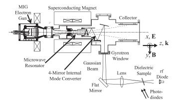
FIG. 1. Schematic of air breakdown experiments. Experiments were conducted with volume and (as shown) dielectric surface breakdown.
