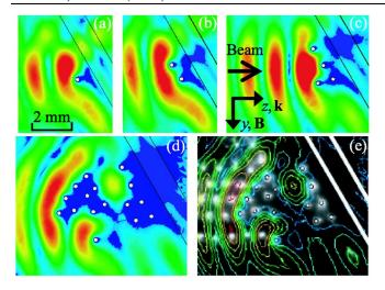
FIG. 6 (color online). Simulations of a filament propagation scenario in a surface breakdown, showing *E*-field magnitude when (a) 1, (b) 2, (c) 4, and (d) 16 filaments exist. (e) Expansion of Fig. 5 with (d) overlaid on top. Scale of (a) also applies to (b)– (e).
