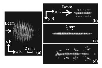
FIG. 3. Typical time-integrated volume breakdown plasma images in (a) E plane and (b)–(d) H plane (camera exposure time  $\gg$  pulse width).
