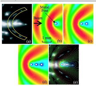
FIG. 4 (color online). (a) Volume breakdown image in the H plane with a crescent region enclosing a curved plasma structure of interest. *E*-field magnitude with (b) 1, (c) 2, and (d) 3 filaments modeled as metal posts (white circles) in the simulations. (e) Superposition of (d) on top of (a).
