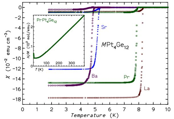
FIG. 1 (color online). Magnetic susceptibility  $\chi(T)$  of filled skutterudites  $\text{MPt}_4\text{Ge}_{12}$  ( $M = \text{Sr}, \text{Ba}, \text{La}, \text{Pr}$ ) for  $\mu_0 H = 2 \text{ mT}$  (nominally). The inset shows the inverse molar susceptibility  $H/M$  of the Pr compound for  $\mu_0 H = 1 \text{ T}$ .
