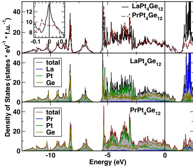
FIG. 4 (color online). Total (upper panel) and atom resolved electronic density of states for  $\text{LaPt}_4\text{Ge}_{12}$  and  $\text{PrPt}_4\text{Ge}_{12}$ . The inset in the upper panel shows the well-pronounced peak in  $\text{LaPt}_4\text{Ge}_{12}$  in a narrow region around the Fermi level.
