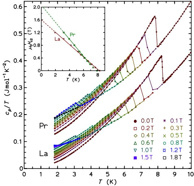
FIG. 2 (color online). Molar specific heat  $c_p/T$  of  $\text{LaPt}_4\text{Ge}_{12}$  and  $\text{PrPt}_4\text{Ge}_{12}$  (shifted upwards by 0.1 units) for different magnetic fields. The inset shows the critical fields  $H_{c2}$  derived from the midpoints of the transitions in  $c_p(T, H)$ .
