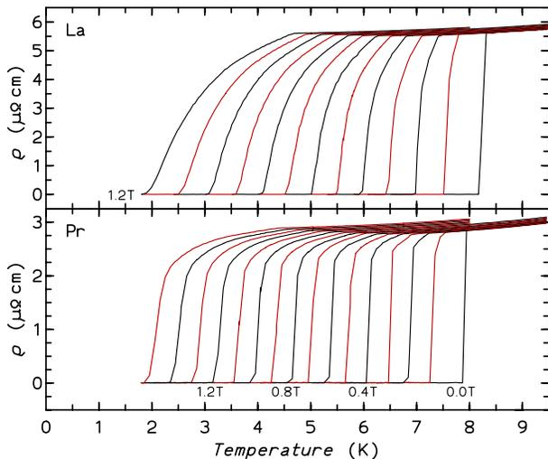
FIG. 3 (color online). Electrical resistivity of  $\text{LaPt}_4\text{Ge}_{12}$  (La) and  $\text{PrPt}_4\text{Ge}_{12}$  (Pr) in magnetic fields with  $\Delta\mu_0 H$  of 0.1 T.
