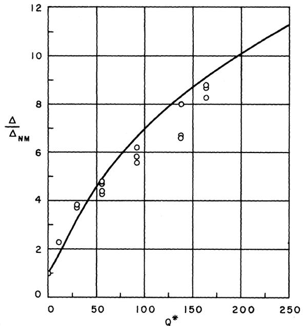
FIG. 2. Experimental data and theoretical curve for the variation of stand-off distance with  $Q^*$  for air. Free stream conditions are  $\rho / \rho_0 = 1.22 \times 10^{-3}$ ,  $T = 6450^\circ\text{K}$ ,  $U = 6890$  m/sec and  $M = 4.5$ .
