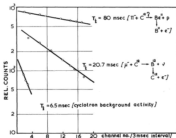
FIG. 2. Decay of the delayed activity at the  $\pi^-$  peak,  $\mu^-$  peak, and with a large absorber.
