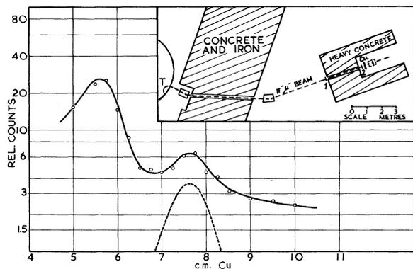
FIG. 1. Experimental arrangement, and absorption curve of activity in the scintillator between the beam pulses of the cyclotron. The dotted curve represents the  $B^{12}$  activity after subtraction of background and  $\pi$ -capture activities.
