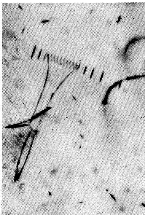
FIG. 1. Generation of prismatic loops from a helical dislocation. The dislocations have been decorated with copper and photographed with infrared sensitive plates. Separation of turns of the helix is about 10 microns.
