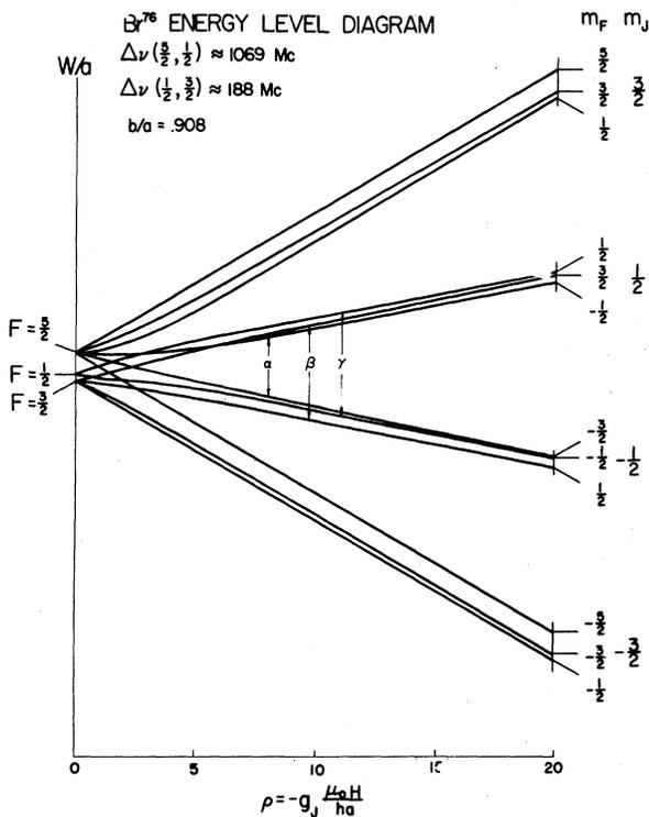
FIG. 2. Br<sup>76</sup> energy-level diagram. This diagram was calculated with an IBM-650 computer, using a  $b/a$  value of 0.908. The hfs separations listed are approximate only.
