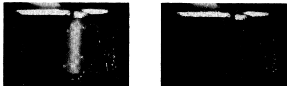
FIG. 1. Photograph of longitudinal sound beam in quartz cube. Frequency \nu = 1000 Mc/sec. In the picture on the right, the HF Power was turned off.
