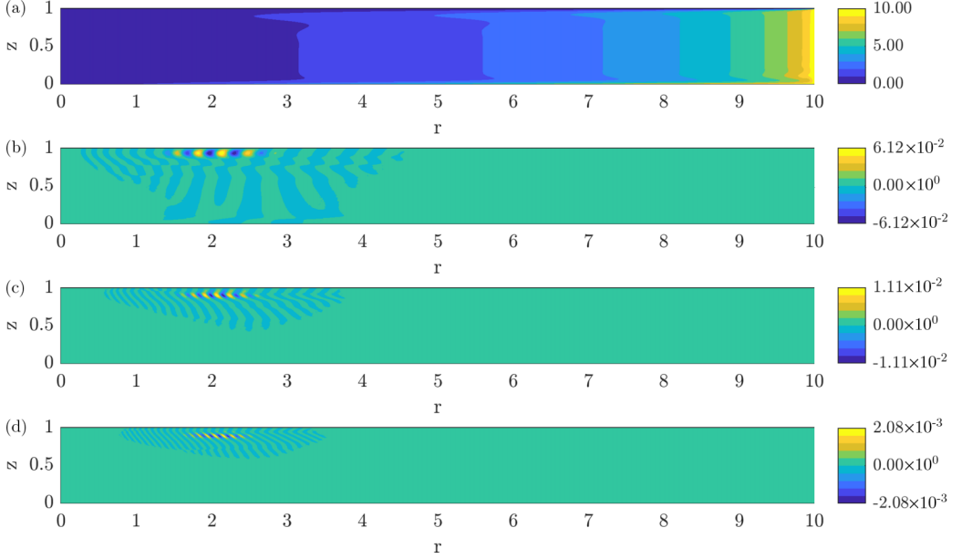
FIG. 10. (a) Contours of U_\theta . (b)–(d) u_\theta for temporal harmonics k = 1, 2, 3 (from top to bottom) for the lower periodic-subcritical solution at \text{Re} = 2300 . Spatial resolution R0 , nt = 3 .
