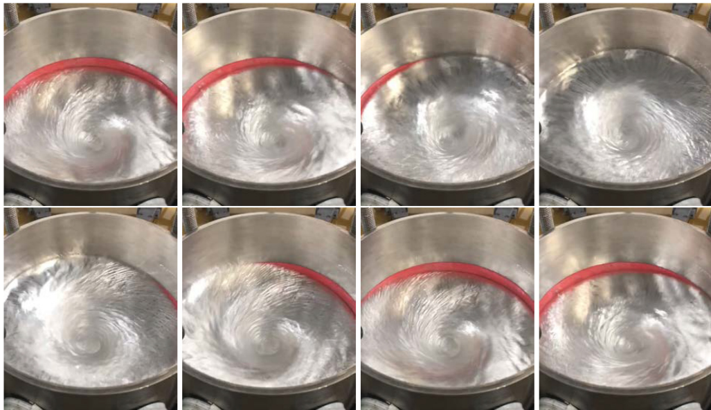
FIG. 3. A sequence of photos of the liquid metal surface in CSW mode taken with a time step \sim 0.067 s (from left to right, from top to bottom). The insulator (colored in red) can be seen in the area of the surface level decrease.
