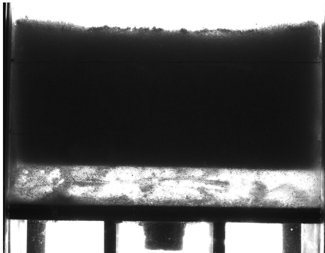
FIG. 6. Example of block uplift for d = 0.7 mm, X_p = 0.1\% , and H = 8 cm.
